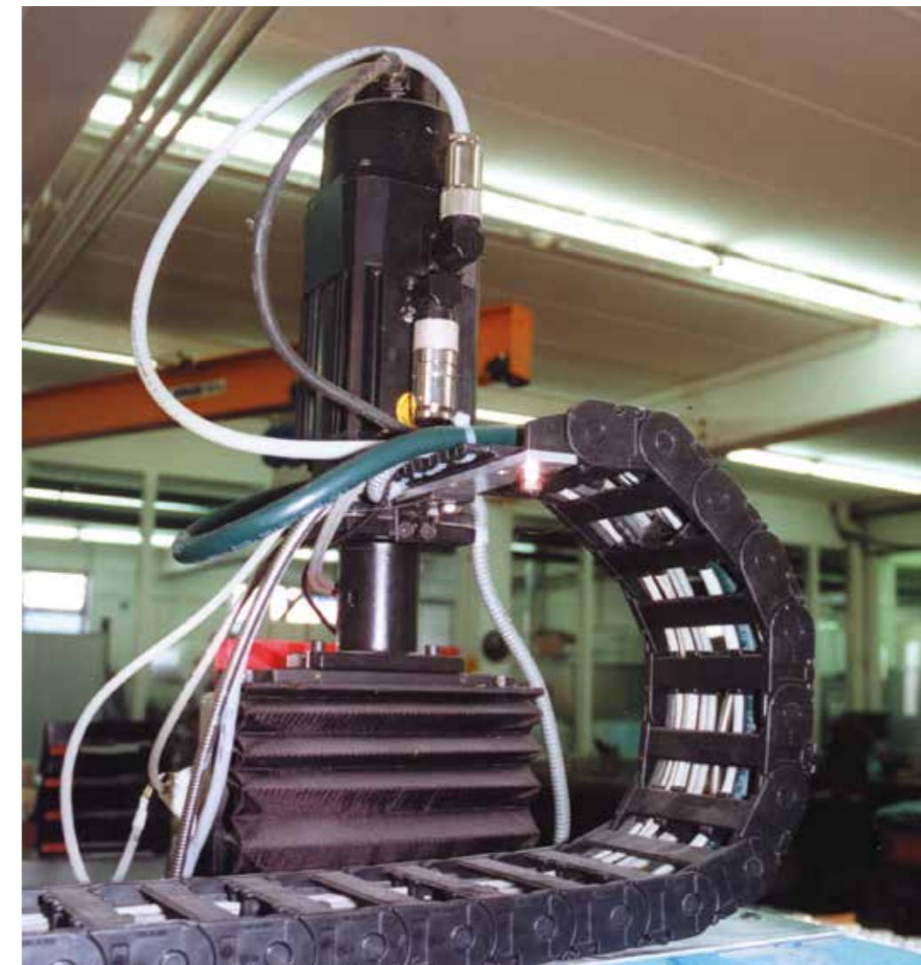
chainflex® CF21.UL: cables for energy supply systems in spinneret production. e-chain®: E2/000
